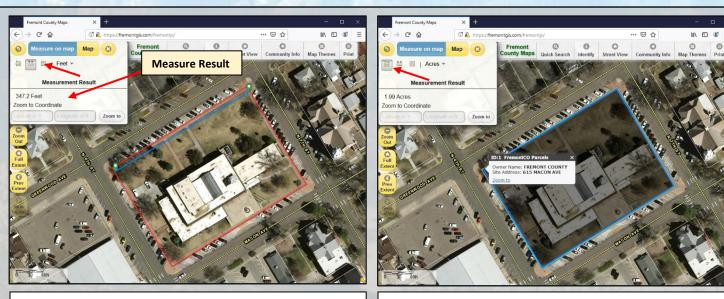
19). To **Measure Distance** select the tool seen above and <u>left click</u> on the point you wish to start your line. The distance of your line will be seen below the **Measure Test Result** field in the Measure Tool. **Double** <u>left click</u> to end your measurement.
