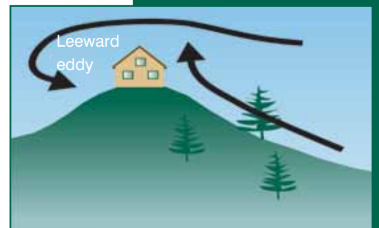
Figure 3-3: Ridge with wind exposure
